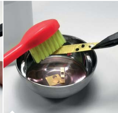
With a brush clean the parts, the acetone will remove all possible traces of grease and dirt.
